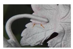
Figure 5. Enlarged view of discovered crack (≈6mm in length) at leaf
