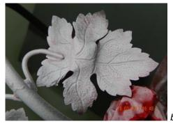
Figure 4. Two stages in penetrant testing after spraying with: a) activator and b) developer
