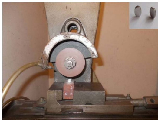
Fig. 3. Preparation of samples for characterization [5]; the inserted image in the upper right corner shows samples of circular cross-section
