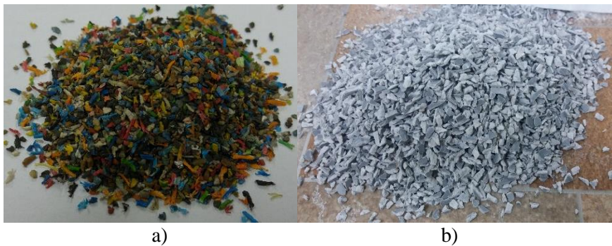
Figure 1 PVC samples a) insulation and b) pipe
