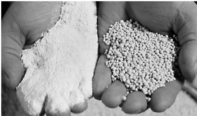
Picture 2. Potash fertilizer before and after pelletizing
