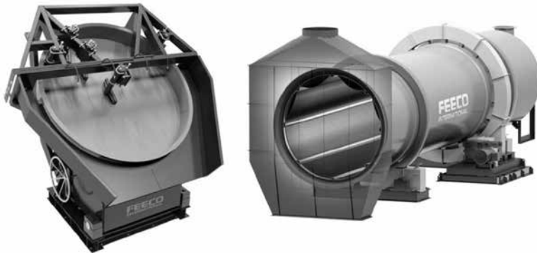
Picture 3. 3D Models of a Disc Pelletizer (left) and Rotary Drum Agglomerator (right)
