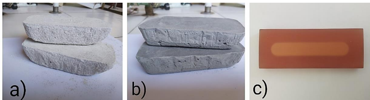
Figure 2. Laboratory samples for testing the release of heavy metals: a) with \text{Ca(OH)}_2 , b) with cement, c) with UPR
