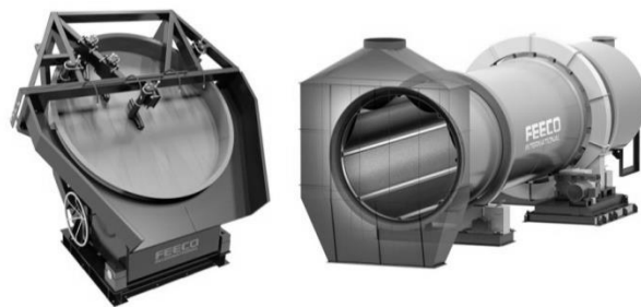
Figure 3 3D Models of a Disc Pelletizer (left) and Rotary Drum Agglomerator (right)
