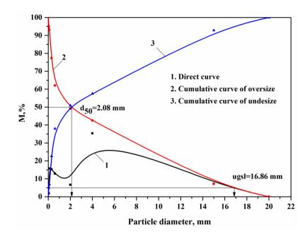
Fig. 1. Curves of the grain size distribution of raw quartz sand "Bijela Stijena"-Skočić.
