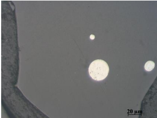
Figure 2. Inclusions of spherical lead alloy in the glass matrix. Reflected light, air, II Nikoli.
